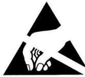
The product contains electronics which may be sensitive to electrostatic discharges (ESD) as well as mechanical stress. To avoid damages, any open circuit board like LED-modules should never be directly touched by hand or by a tool.
