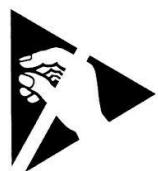
The product contains electronics which may be sensitive to electrostatic discharges (ESD) as well as mechanical stress. To avoid damages, any open circuit board like LED-modules should never be directly touched by hand or by a tool.
